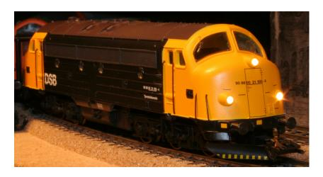
Märklin DSB MY 118 (The yellow locomotive) comes with a Delta module. This means you cannot control the headlights and the locomotive address can only be set on dip-switches removing the locomotive haul.
